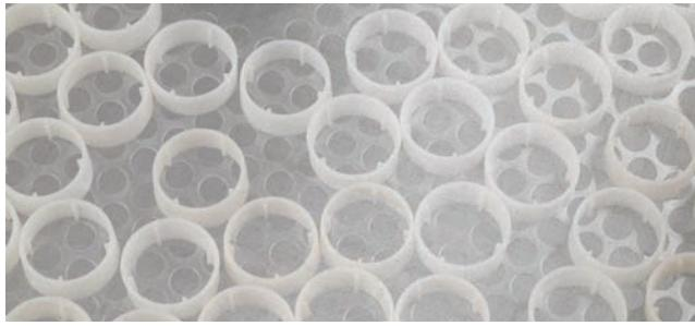
**Antiblending devices, like the sliders shown here, help prevent particles from sticking in the screen openings.**
